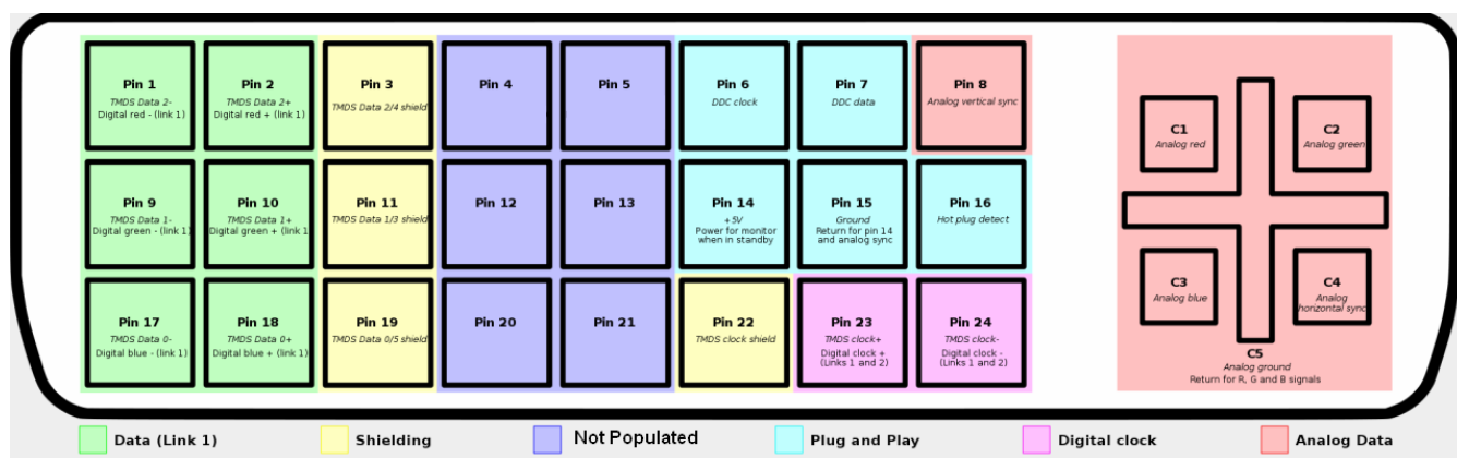
Figure 5.3 PROTON-LVDS DVI-I Single Link (input and output).
